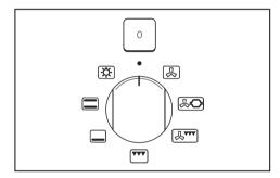
Turn the programme dial clockwise or anti-clockwise to the required programme position.
